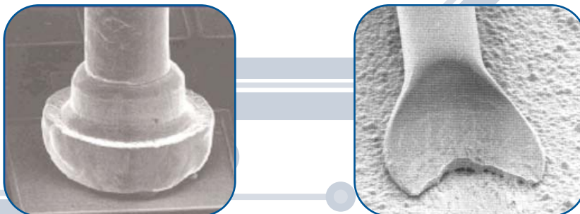
Figure 1: Typical First & Second Bond Morphology of X-Wire
