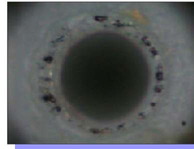
Negligible Build Up in Capillary Wall Observed
