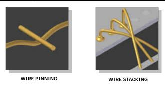
Fig. 8: Examples of future layouts of insulated bonding wire, defined as wire pinning and stacking.
