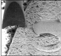
Fig. 4: Example of acceptable stitch bond strength for insulated bonding wire, after peel test. Wire bonding courtesy of ASM Pacific.
