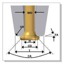
Fig. 5: Capillary Dimensions. Source: SPT
