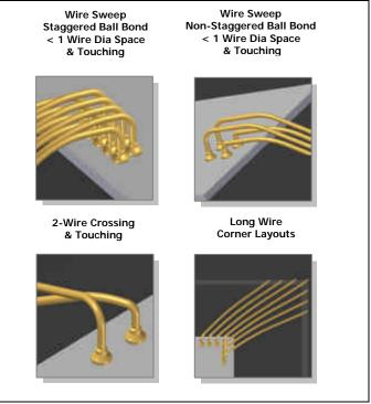
Fig. 7: Example layouts and design rules for acceptable insulated bonding wire packages.
